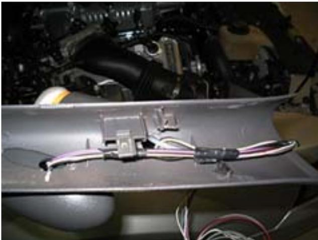
The pillar's "bullets" are designed to house 2 1/16" gauges. Autometer is the brand of choice at Speed of Sound, and exhibit a perfect fit. Should your gauge require a more snug fit, simply attach a small piece of Velcro (only one side, hook or loop, about the size of half a postage stamp) or a single wrap of electric tape at the rear of the gauge. This will ensure a firm fit.
