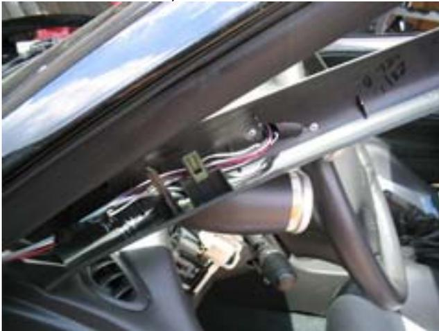
For best results, align the new pillar starting from the end closest to the dashboard. Check and correct as needed any slack wiring/tubing as you fit the pillar into place. Insert the lower guide pin and clip into place, pressing lightly to lock it into its attachment point. Now, move the upper clip into position. Once both clips are aligned press firmly to seat the clips to their original fit.
